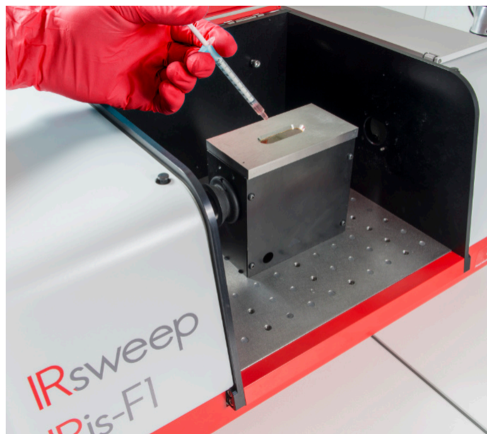
The IRis-F1 dual-comb spectrometer, with its large sample compartment
